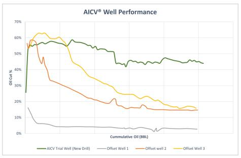
AICV® well performance in the retrofit well demonstrated improved Oil Cut with 45% less water production. Productivity Index (PI) is now better controlled in the water-swept reservoir.
